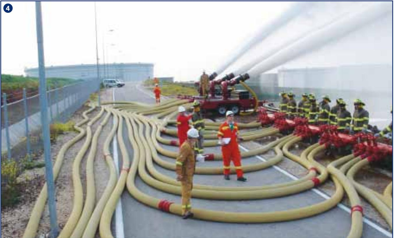
**(4) Large-volume monitors and large-diameter hose are required to battle a large tank fire.**
